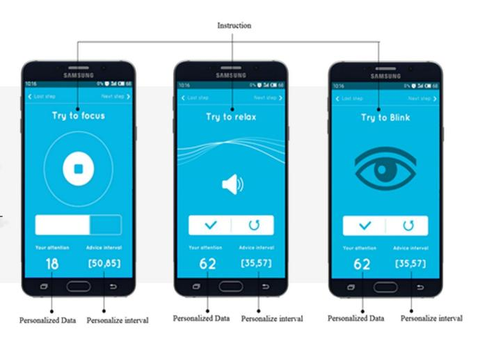
After users set the personalized data, the page of all the data are shown in Figure 6. We design two tasks in this APP so that users can choose the situations to control the Lego robot. Every user can keep or change their own constrains. Final, press the "enter" button then you can start to control the Lego Robot with personalized brain waves.
